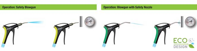
Flow stopped completely and pressure reduced to 0.5 bar Flow diverted and pressure reduced to 0.5 bar
